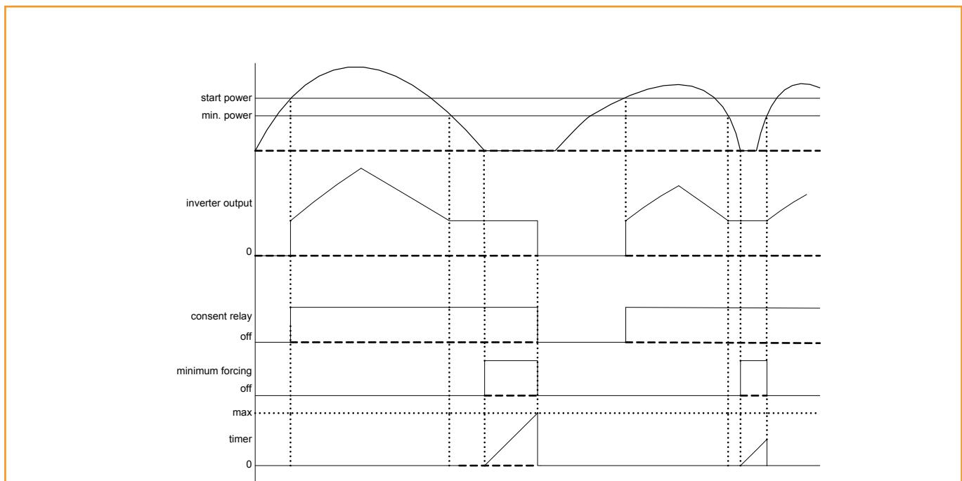
During minimum forcing if temperature or pressure drops below the limit **154-InLPt** inverter output, relay consent, timer and minimum forcing will be forced to zero.
