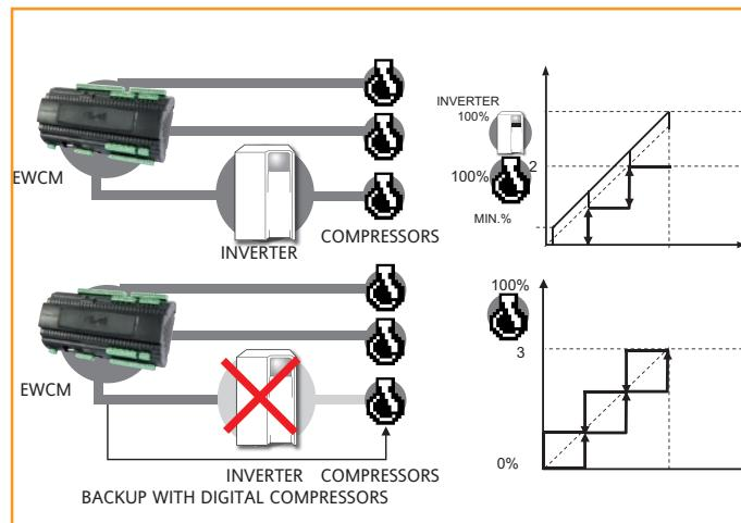
In these cases control is automatically switched to digital compressors.
