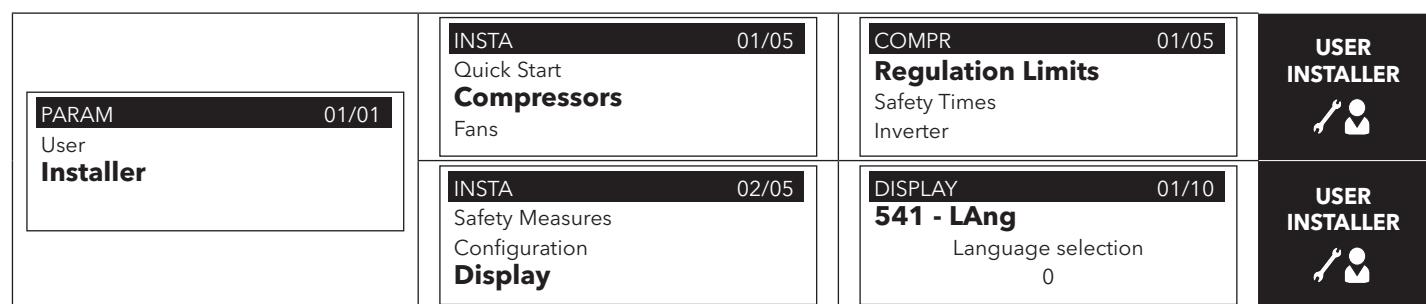
Select the Quick Start folder with 'UP' and 'DOWN' and press 'OK'
