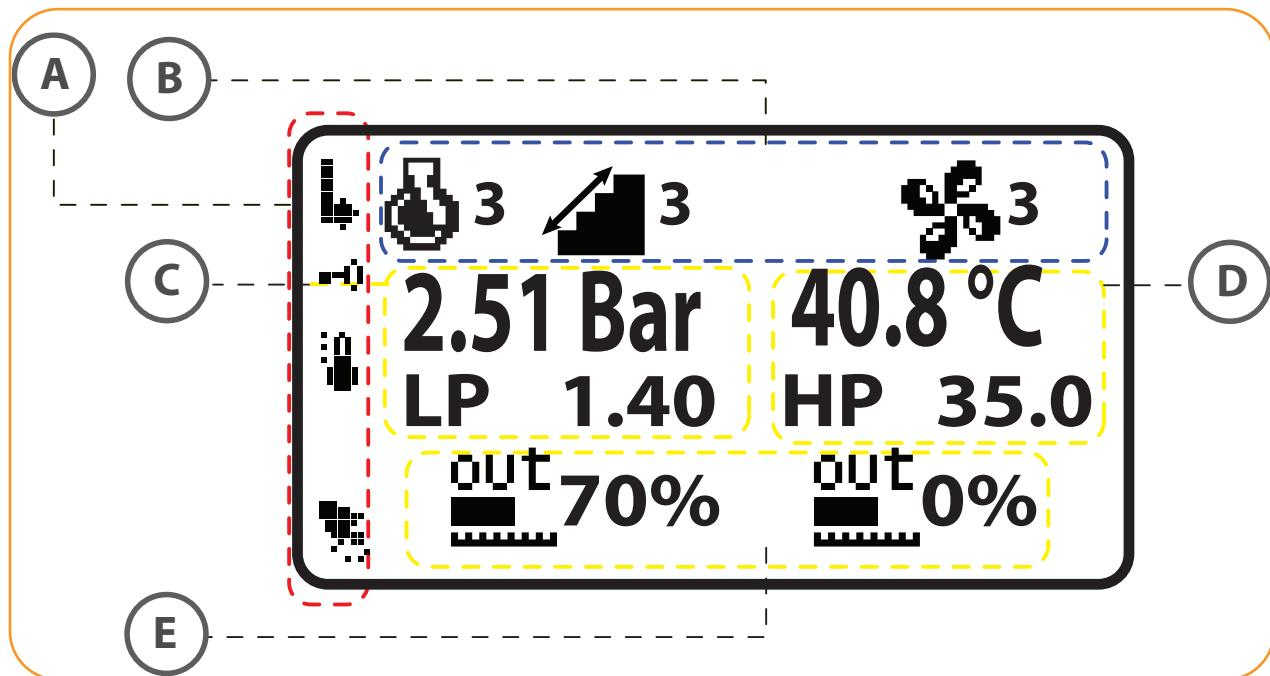
The display is used to monitor the parameters, machine status and operating modes, as well as configuring machine parameters.
