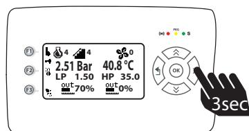
This Menu displays the values of pressure transducers and probes in the plant.
