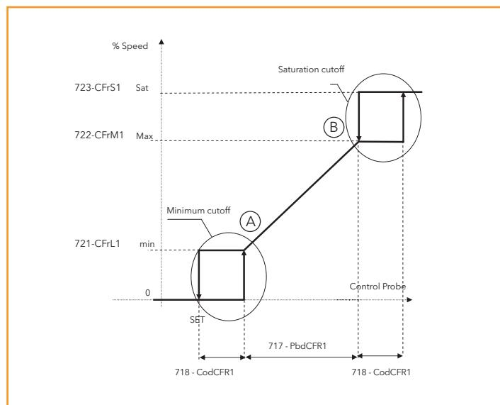
With an analogue output you can set the proportional band **717-PbdCFr1** and minimum actuation percentages **721-CFrL1** maximum **722-CFrM1** and saturation **723-CFrS1**.
