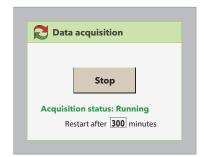
It is useful to set automatic acquisition restart, to prevent the user from inadvertently leaving data acquisition off following maintenance work.
