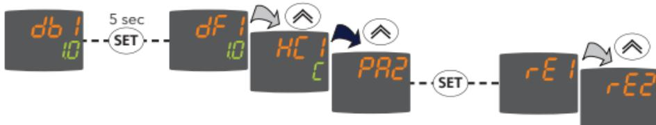
Press the **set** key next to the desired folder ("rE2" in the example), the first parameter contained in the folder will be displayed. Select the desired parameter using the **↑** and **↓** keys. Change the value (shown on the second line) using the **↑** and **↓** keys, then press the **set** or **fnc** keys to store the new value.
