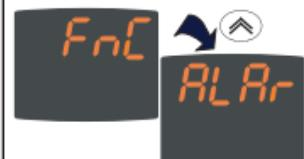
After pressing the **fnc** key, you can scroll through the two folders in the menu (FnC and ALAr) using the and keys.
