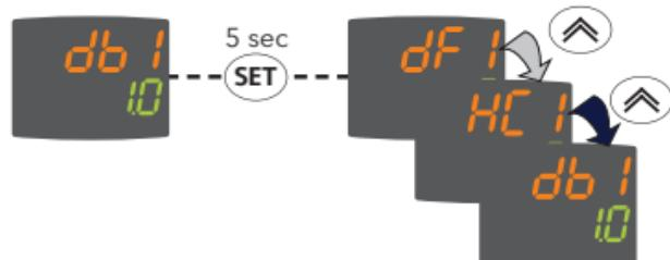
Select the desired parameter using the **▲** and **▼** keys.
