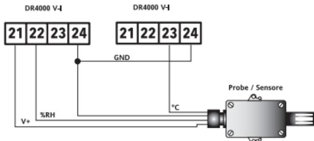
**CAUTION:** wire colours are guideline. Check the correct connection diagram on the probe label.
