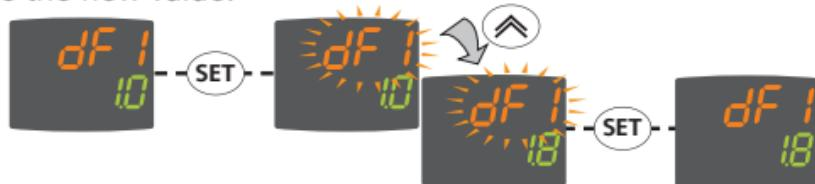
**NOTE:** It is advisable to switch the instrument off then back on again each time parameters are modified to prevent malfunction of the configuration and/or timer operations underway.
