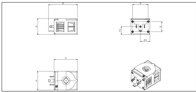
Fig. 15. coil mechanical dimensions models PXVB0ARA60100, PXVB0ARA20100
