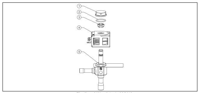
**Fig. 7.** 8 W coil, body 03/M10
