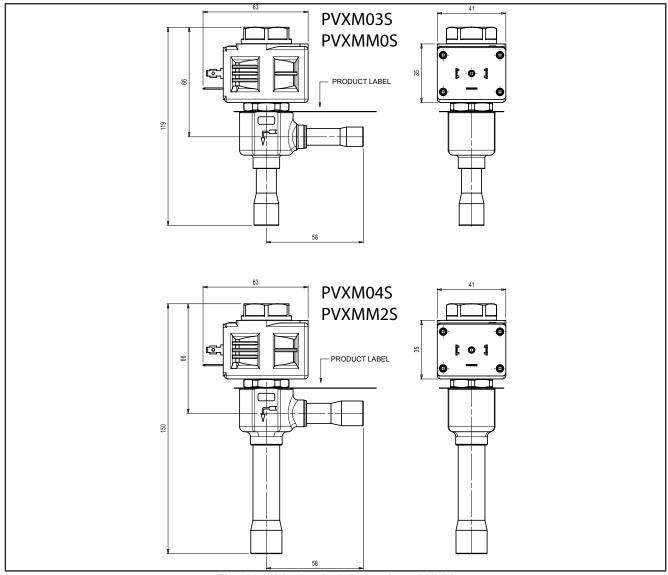
Fig. 13. Mechanical dimensions PXVM
