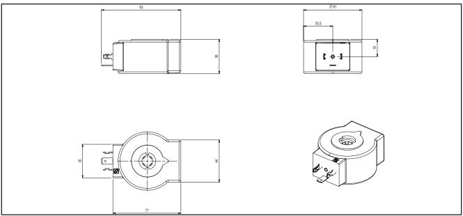
Fig. 14. coil mechanical dimensions for models PXVE0ARA60100, PXVS0ARA60100
