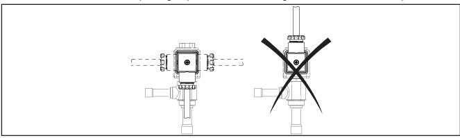
Fig. 11. Connector positioning
