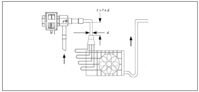
Fig. 4. Detail Valves and evaporator
