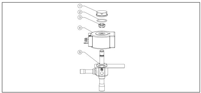
**Fig. 8.** 12 W coil body 03/M10
