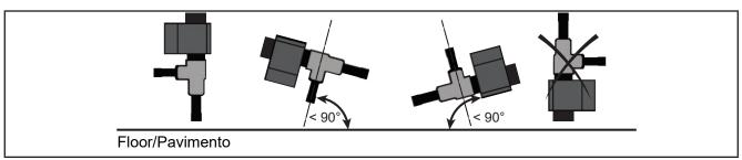
Fig. 2. Valve positioning
