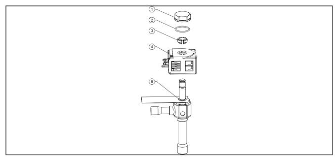
**Fig. 9.** 8 W coil, 04/M12 body
