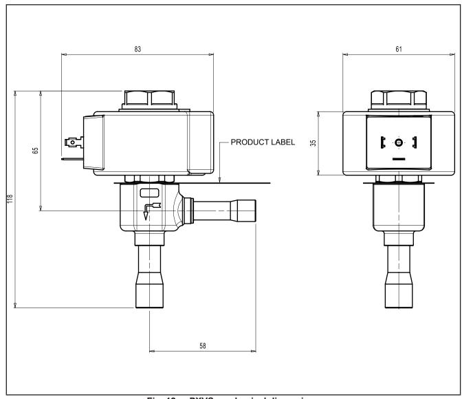
Fig. 12. PXVS mechanical dimensions
