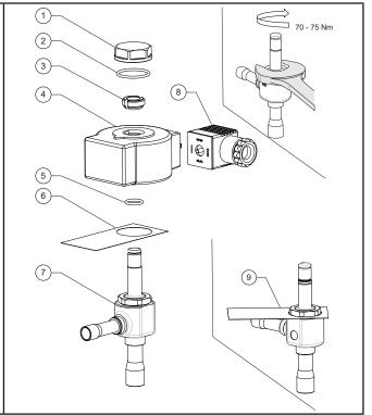
Fig. 6. Valve coil and connector components
