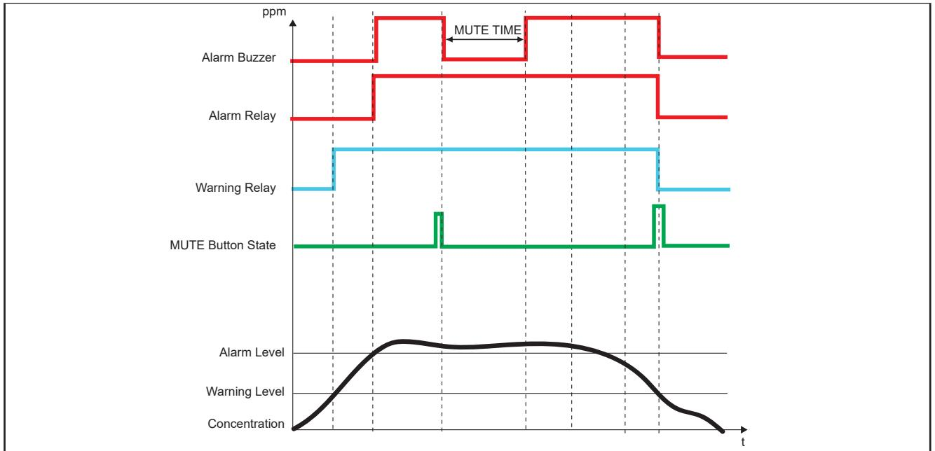
**Fig. 24.** Alarm/Warning sequences
