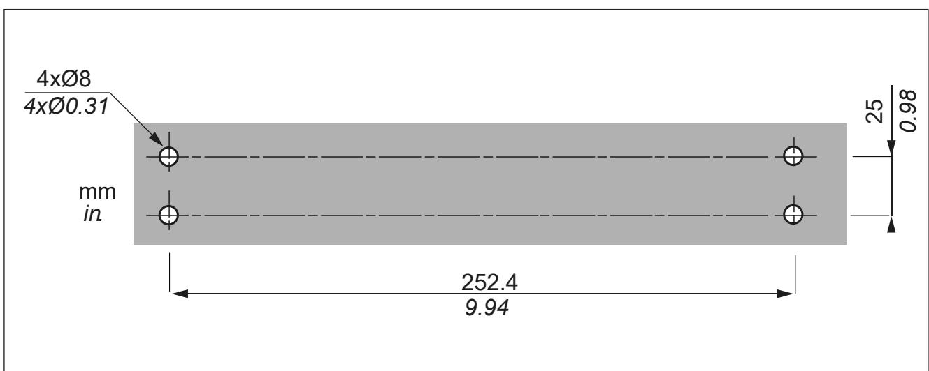
Use 6 mm (0.23 in.) diameter screws and tighten to 8.5 Nm (75.23 lb-in.).
