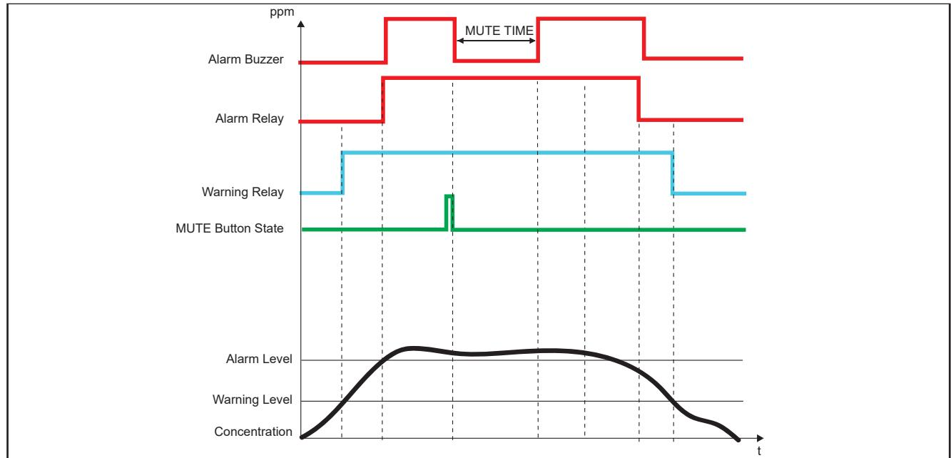
**Fig. 23. Alarm/Warning sequences**
