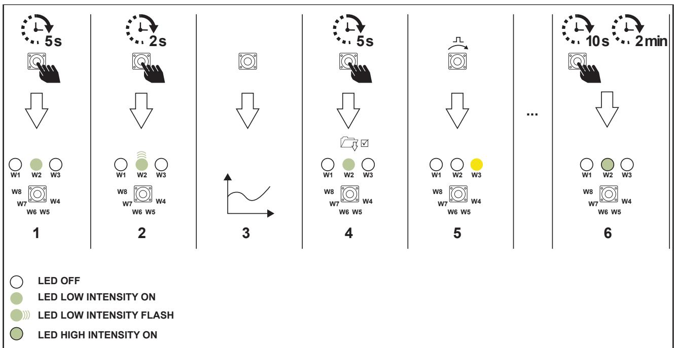
Fig. 21. Service Wheel procedure
