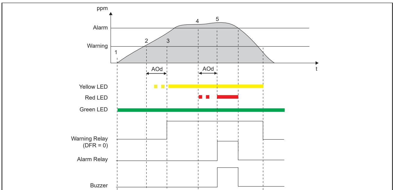
Fig. 22. Alarm/Warning sequences
