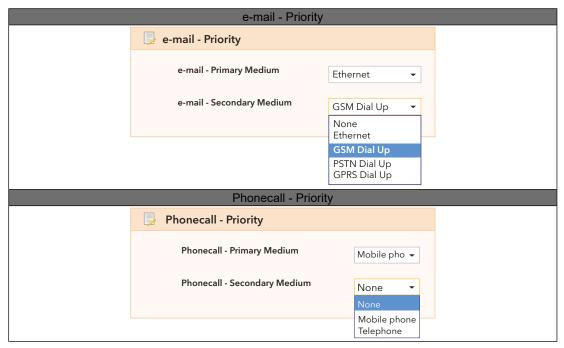
For example, in the e-mail Priority box you can select the primary medium for sending alarm notifications via email (Ethernet, in the example shown). If the Ethernet connection is not available, the Televis**Go** will attempt to send emails using the secondary medium (in this case a GSM modem).
