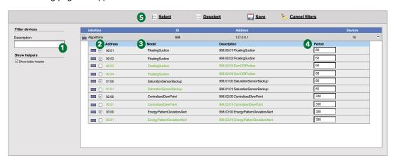
This screen shows the list of algorithms previously loaded within the TelevisGo (see "12.1. SYSTEM UPDATING" on page 115) and the corresponding settings.
