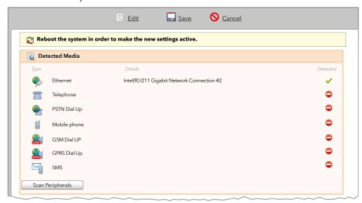
The Detected Media box lists the elements found, plus the corresponding connection **type**. The column **Detected** indicates whether the specified medium has been detected, while the column **Details** shows its description.
