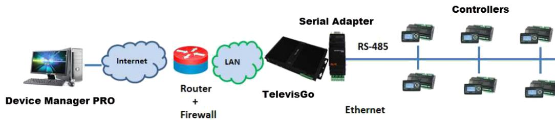
This connection method uses the proprietary TelevisSerialAdapter protocol. For instructions on how to set up this connection, see Set up communication with the controller.
