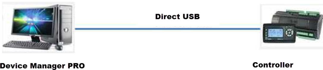
This connection method uses the Modbus protocol. For instructions on how to set up this connection, see Set up communication with the controller.
