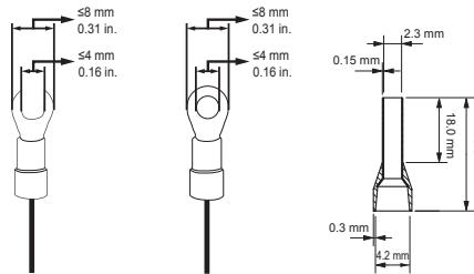
Wire using cable lugs, ferrules or bare conductor.
