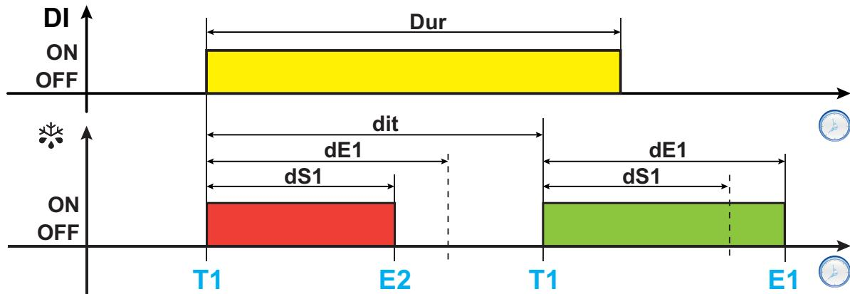
**Legend:** Dur = DI Duration; DI = Digital Input; = Defrost; T1 = Defrost request; T2 = Regular defrost request with fixed expiration; E1 = Defrost end due to timeout; E2 = Defrost end due to temperature.
