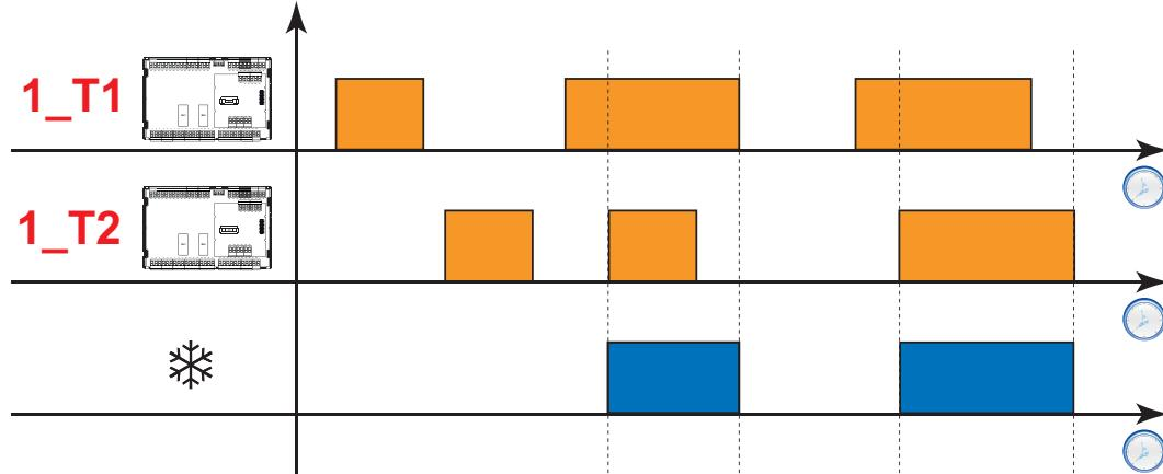
**Legend:** **1\_T1** represents the progress of the probe set as thermostat 1 and **1\_T2** represents the progress of the probe set as thermostat 2.
