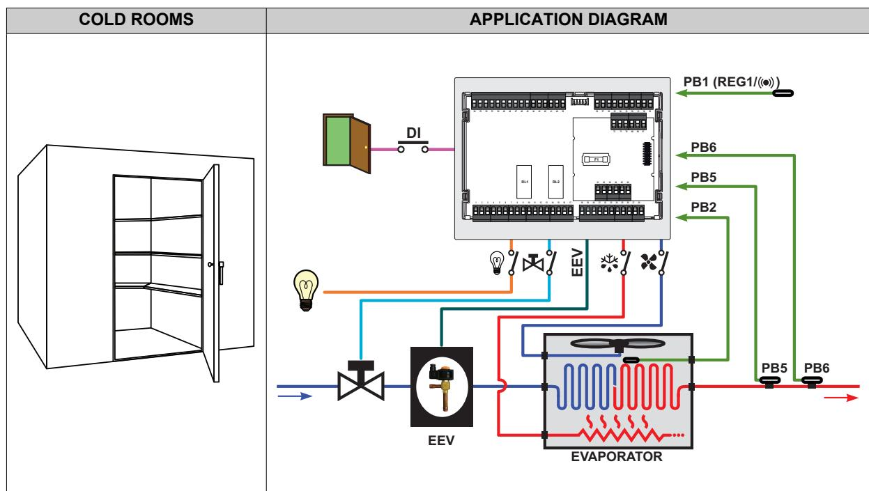
Legend: **REG1** = Regulator 1; **EEV** = Electronic expansion valve; **Evaporator** = Evaporator.
