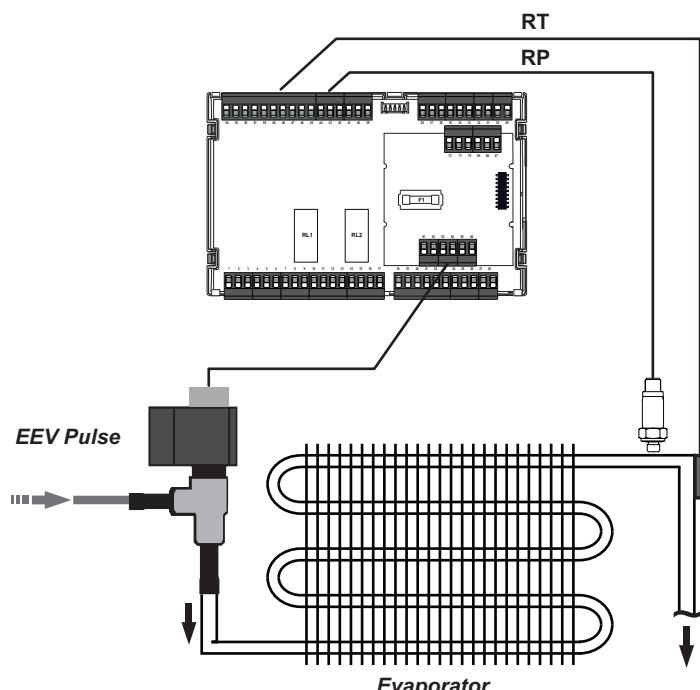
**Legend:** **RT** = Refrigerant Temperature; **RP** = Refrigerant Pressure; **EEV Pulse** = Pulse Valve; **Evaporator** = Evaporator.
