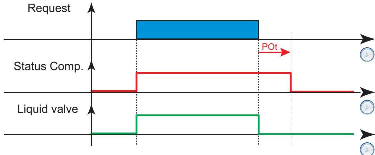
Legend: **Request** = Request cooling; **Status Comp.** = Compressor Status; **Liquid valve** = Liquid valve.
