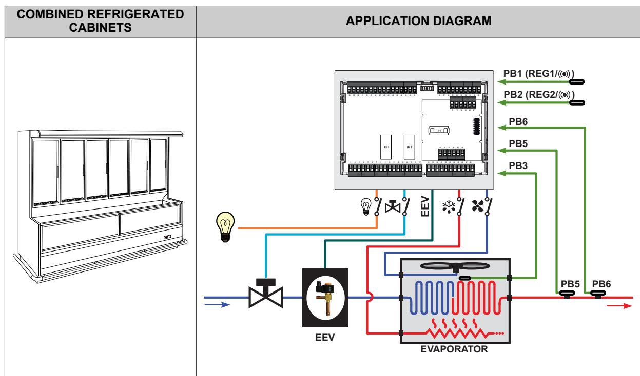
**Legend:** REG1/2 = Regulator 1/2; EEV = Electronic expansion valve; Evaporator = Evaporator.
