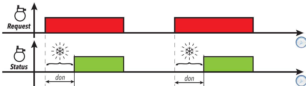
**Legend:** PO = Controller switch-on; = Compressor icon flashing; **Request** = Compressor activation request; **Status** = Compressor status (ON/OFF).
