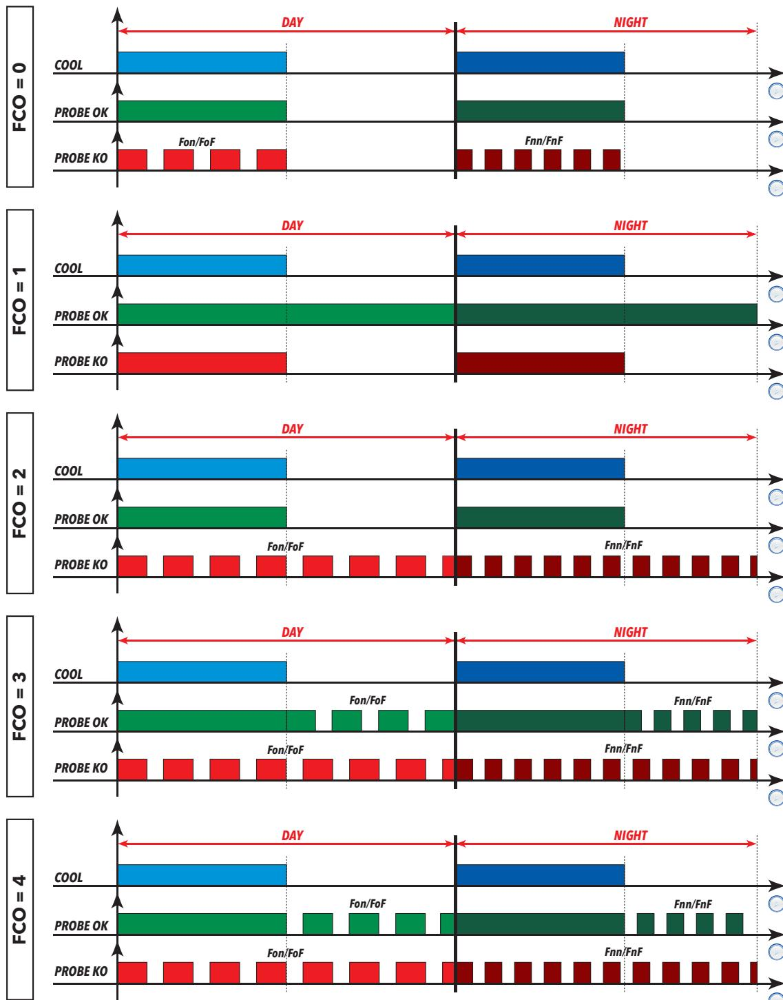
**Legend:** **DAY** = Day; **NIGHT** = Night; **COOL** = Cooling; **Probe OK** = Fan operation with probe present and working; **Probe KO** = Fan operation with probe present but in error.
