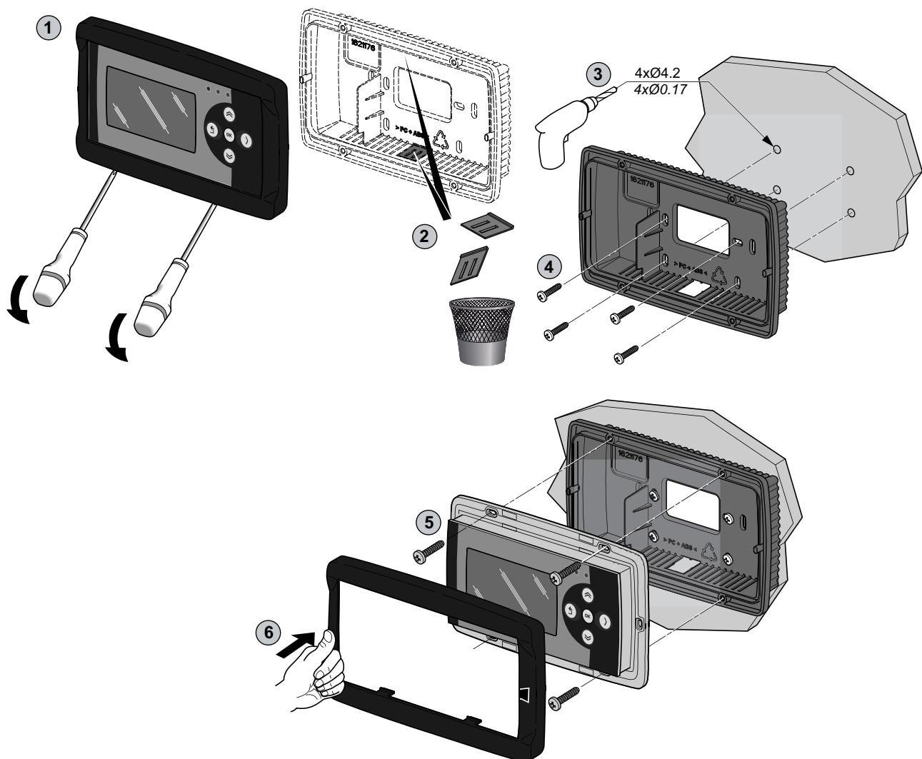
The following procedure explain how to install AVK1000000500 remote display on a vertical surface:
