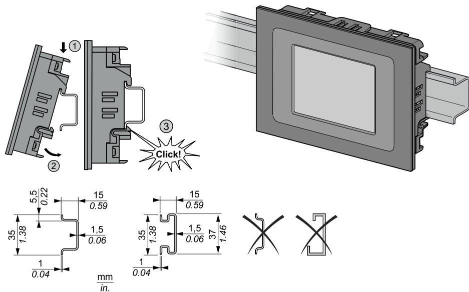
The following procedure describes how to install a AVP100•OP0500 remote display on a top hat section rail (DIN rail):
