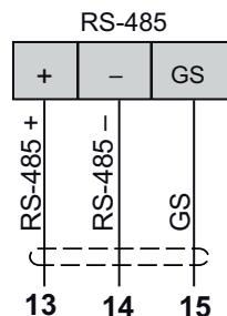
**NOTE:** GS of the RS-485 terminal is not internally connected to the “-” of the power supply terminal of the device.
