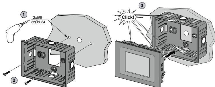
The following procedure explain how to install AVP100•OP0500 remote display on a vertical surface:
