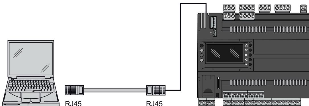
To connect the PC to the controller, use a RJ45 Ethernet cable.
