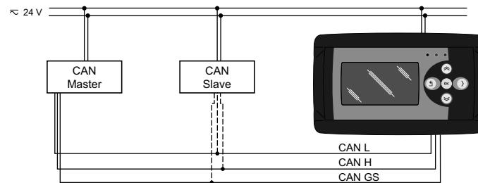
**NOTE:** Both ends of the CAN expansion bus must be terminated. In AVK1000000500, this is possible via its termination jumpers.
