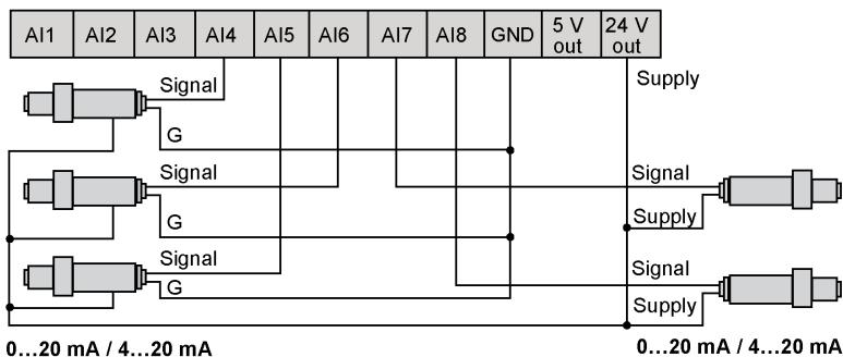
You can power the transducer from the FREE Advance (5 Vdc or 24 Vdc) or with an external supply.
