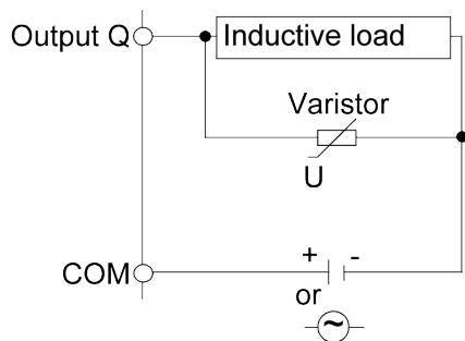
In applications where the inductive load is switched on and off frequently and/or rapidly, verify that the continuous energy rating (J) of the varistor exceeds the peak load energy by 20 % or more.
