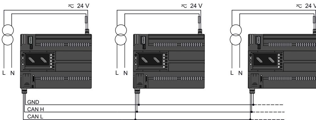
CAN network example with common power line and GND signal not connected:
