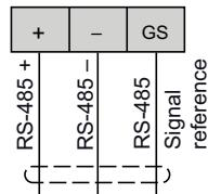
**NOTE:** GS of the **RS485-1** and **RS485-2** terminals are internally connected and are isolated from the GND of the device.
