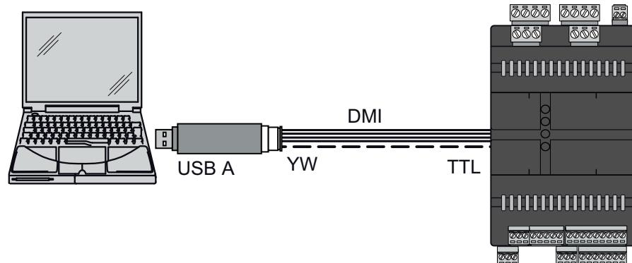
To connect the PC to the expansion module, use a DMI programming cable (Yellow) on the TTL port of the device.
