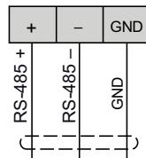
**NOTE:** GND of the **RS485-1** and **RS485-2** terminals are internally connected to the GND of the device.
