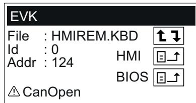
If occurs, check the communication configuration of the remote display, page 122 and the communication wiring, page 118.
