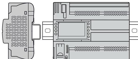
AVC840006I500 / AVD840006I500 / AVD84SS06I500 / AVC126006I500 / AVD126006I500 / AVD126S06I500 controllers can be mounted vertically or horizontally upward.
