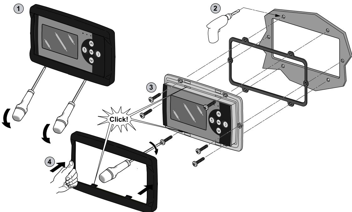
The following procedure explain how to install a AVK1000000500 remote display on a panel:
