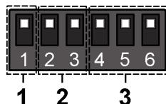
**NOTE:** The addressing comprises the sum of parameter *Addr\_CAN\_OB* (Default value: 1) plus the composite value of the 6-position DIP switches DIP4...DIP6 (8 addresses).
