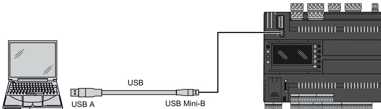
To connect the PC to the controller, use a type A / type Mini-B USB cable.
