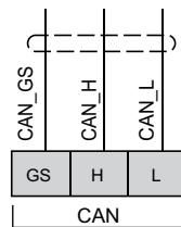
**NOTE:** The terminals of power supply connection and the signal reference for CAN Expansion Bus (indicated as GS) are not internally connected.
