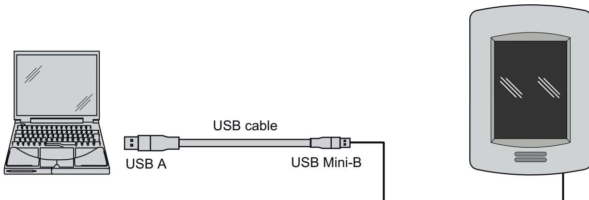
To connect the PC to the remote display, use a type A / type micro-B USB cable.
