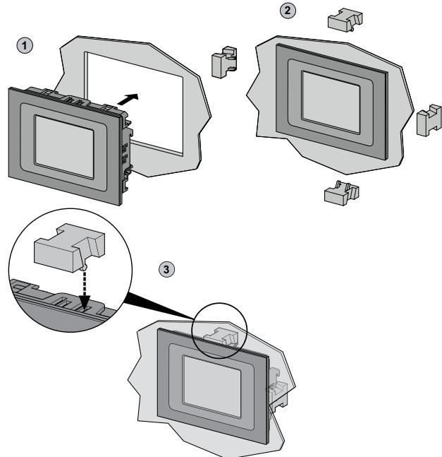
The following procedure explain how to install a AVP100•0P0500 remote display on a panel:
