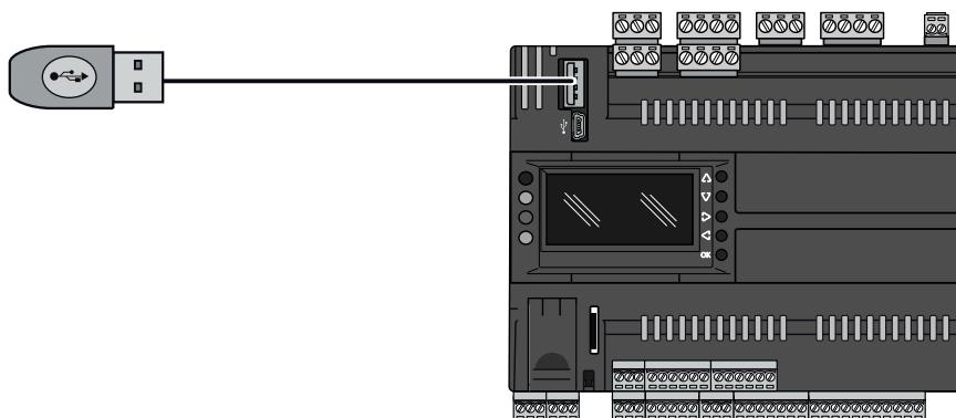
The USB memory key is connected on the type A USB port of the controller.
