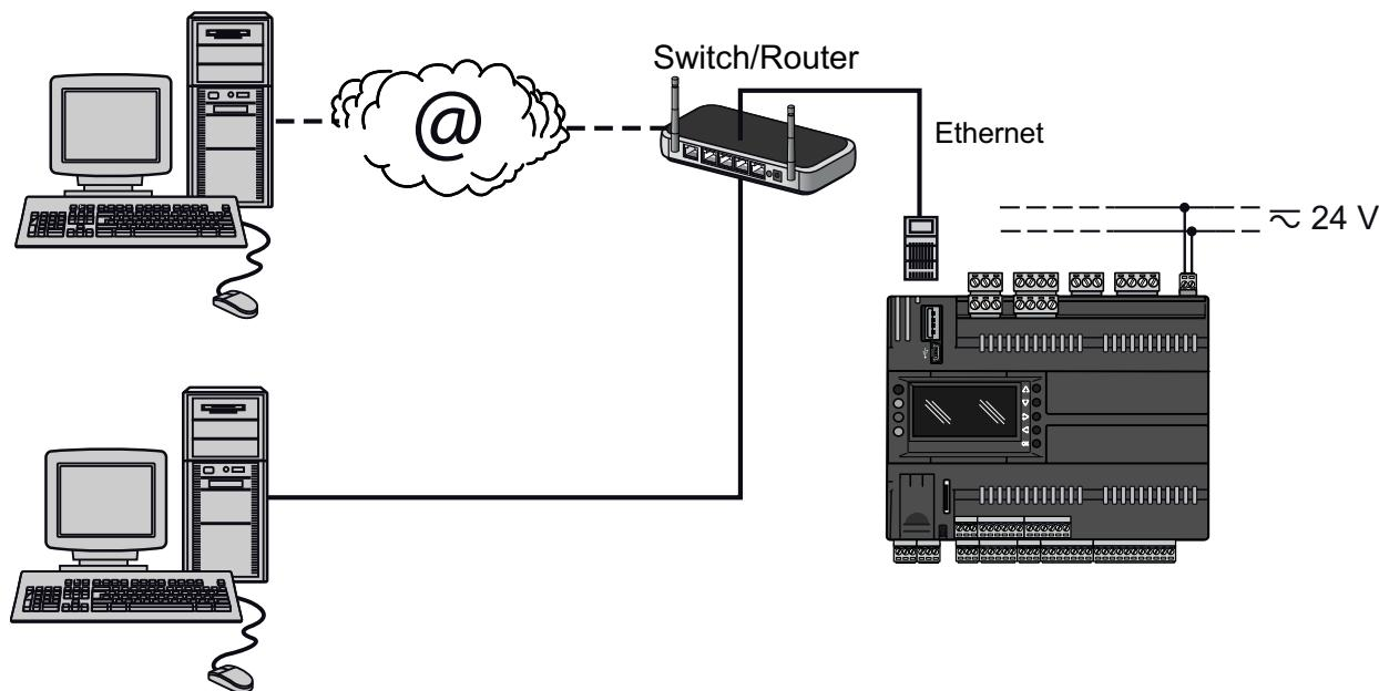
The following diagram shows a BACnet/IP architecture wiring example:
