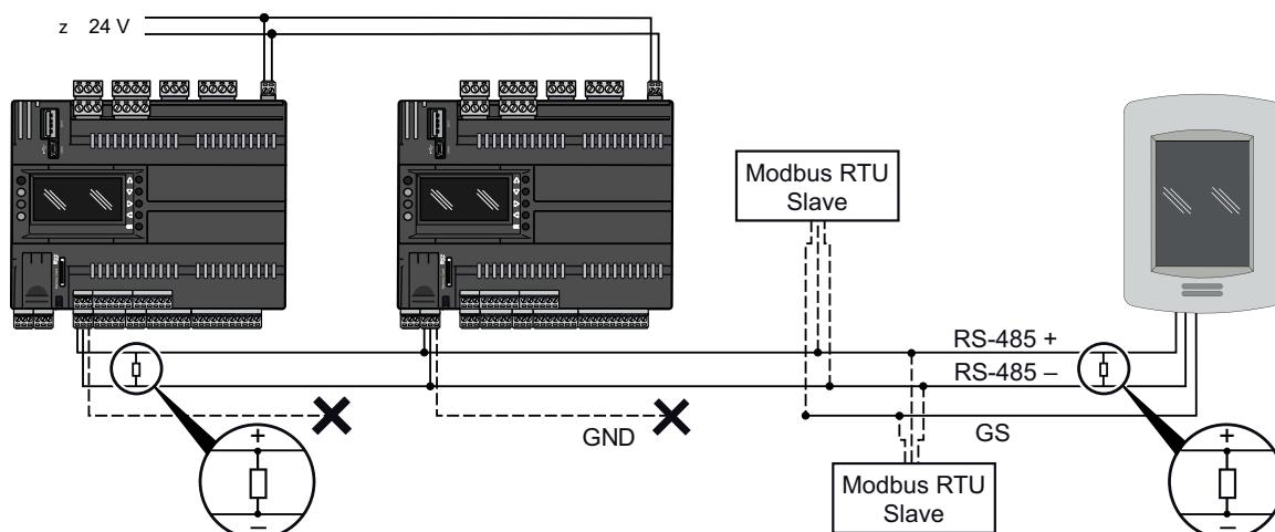
The following diagram shows an RS-485 (field) architecture wiring example with isolated controllers:
