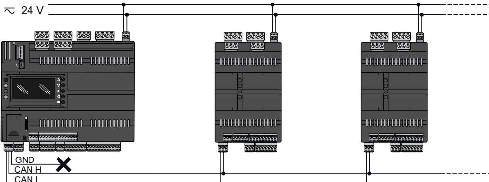
Isolated power supply connection example using a AVD126006I500:
