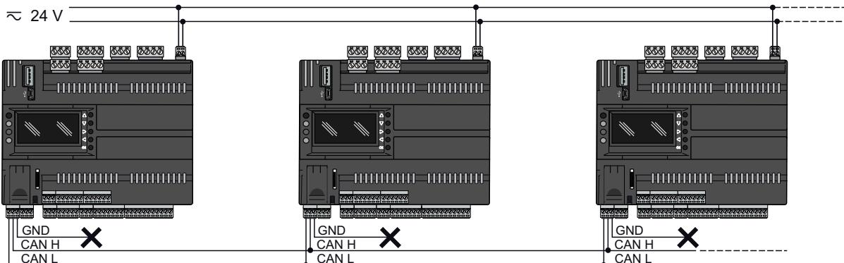
Isolated power supply connection example using AVD126006I500:
