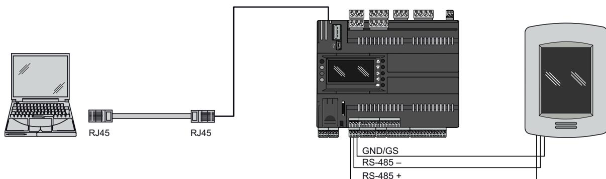
To connect the PC to the AVP1•0...0500 remote display through a controller, use:
