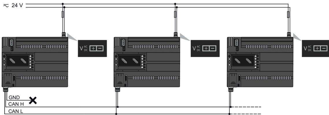
**NOTE:** AV•30...•60500 / AV•62...•0500 / AV•840005I500 / AV•126005I500 / AV•84...•6I500 / AV•126...•I500 power supply inputs are isolated. GS connection of the RS-485 network or the GND connection of the CAN expansion bus across multiple controllers must be connected regardless of the power supply type and wiring.
