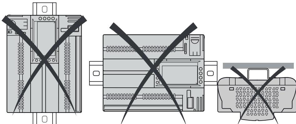
AVD84SS060500 / AVD126S060500 controllers cannot be mounted horizontally upward:
