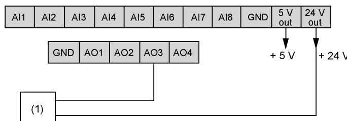
(1) Third-party actuator (for example: fan module) or external relay
