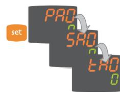
• When the Set key is pressed on the ALAr folder, the first parameter in the folder is displayed, as follows:
