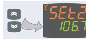
③ The UP and DOWN keys can be used to change the Setpoint value shown on the SV display.
