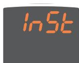
• Indicated by label InSt the UP and DOWN keys can be used to display the InSt label, which indicates the access point of the folders containing the installer level parameters. When InSt is displayed, press and release the Set key
