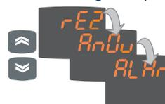
• Press the UP and DOWN keys to scroll through all the user level folders and, on the desired folder, press the Set key to access the parameters in the folder (for example, the ALAr folder).
