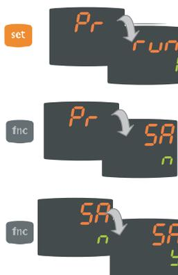
Press the Set key on the desired subfolder to access the parameters. To scroll through the parameters, use the Set key, and to change a value, use the UP and DOWN keys.
