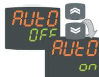
To change the status of a function, use the UP and DOWN keys.
