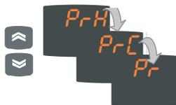
Press the Set key on the Pid label the label of the first subfolder PrH is displayed. Scroll through the subfolders using the UP and DOWN keys.
