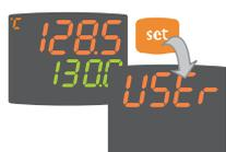
• When the Set is pressed on the main display for 3 seconds, the user can access the Parameter Programming menu; the USER label appears, to indicate user level of the menu.
