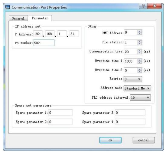
If select "Extended Mode" for Address Mode, settings of IP address and port number here are invalid, while they can be set via the function button "Slave
