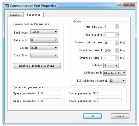
Figure 8-19 Parameter setting page of remote HMI communication port attribute setting
