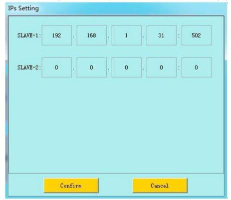
After the above settings, download the project into HMI; connect the master and slave station directly or through a router in order to perform operations of monitoring and control.
