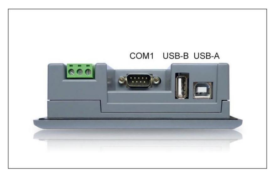
Figure 1-15 Side panels of SK ( single serial )
