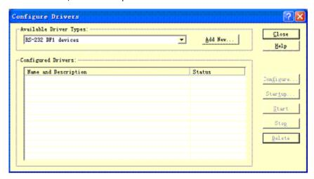
After the settings, the PLC device is available in RSLinx if there is a cable connecting PC and PLC
