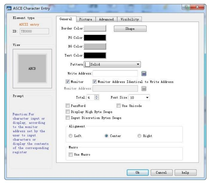
Figure 4-100 ASCII Input dialog box
