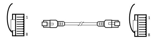
Terminal of HMI is RJ45, and that of Modbus device is RJ45.
