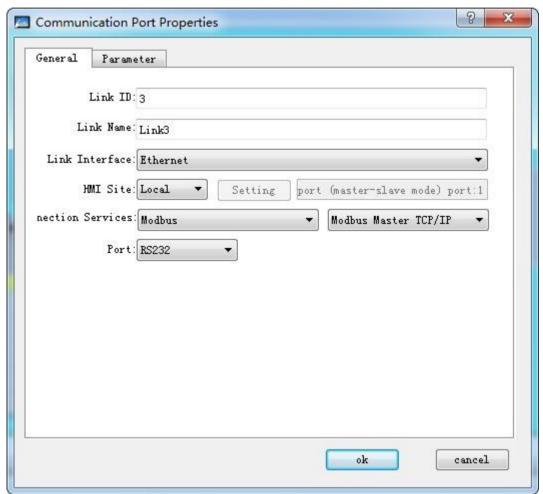
Click "Parameter" in the pop-up "Port Properties" dialog box, enter the following dialog box to set the IP address and the port number (IP address and port are those of monitoring device). Choose standard address mode; Click "OK" to complete the settings.
