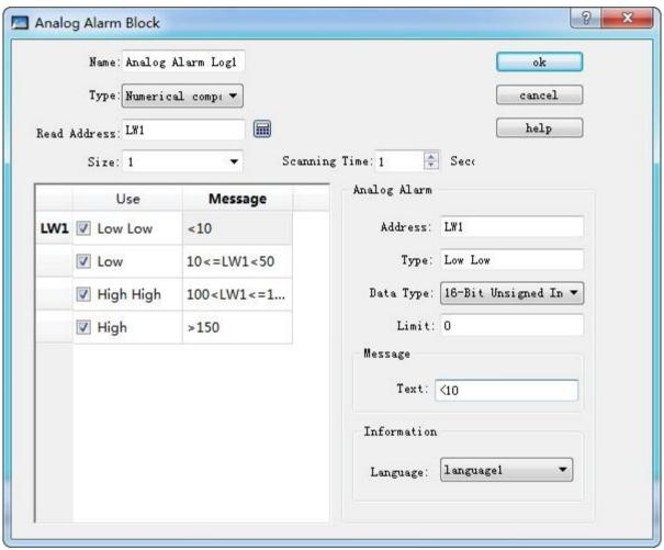
Figure 7-28 Analog Alarm Login dialog box
