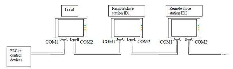
Figure 8-13 Sketch map of penetration connection involving multiple screens
