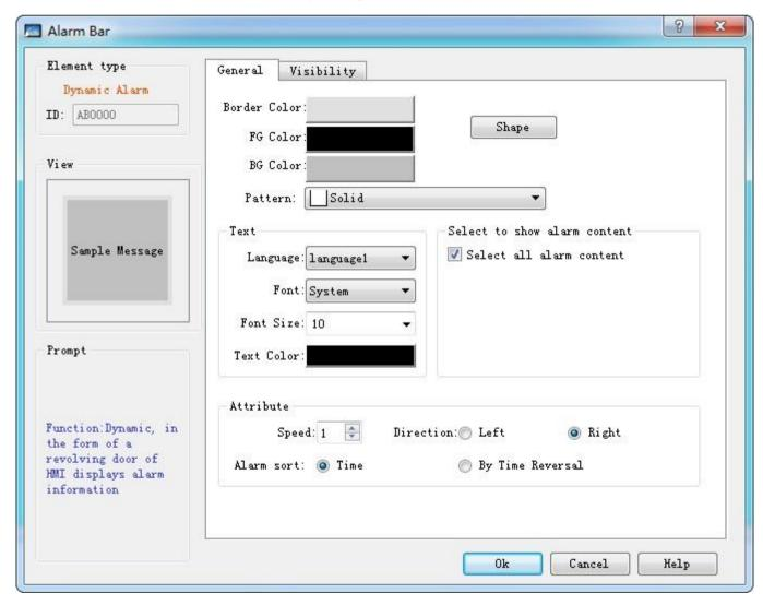
Figure 7-27 Dynamic Alarm Bar Properties dialog box
