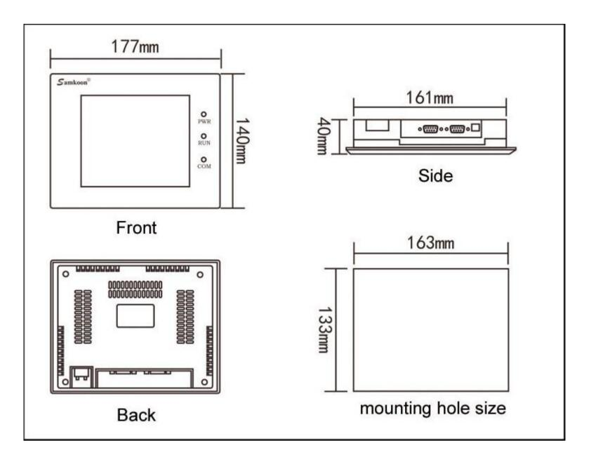
Figure 1-5SK-057FE mounting dimension
