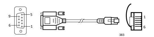
Terminal of HMI is DB9F, and that of Koyo SN series PLC is 6-pin registered jack.
