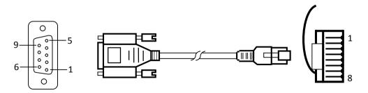
Terminal of SK HMI is DB9F, and that of Fuji NB series PLC is RJ45.
