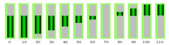
Figure 4-103 bipolar bar graph
