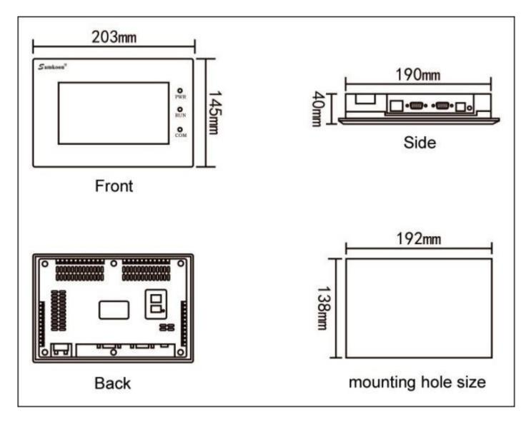
Figure 1-7 SK-070H mounting dimension
