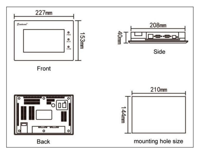
Figure 1-6 SK-070F mounting dimension
