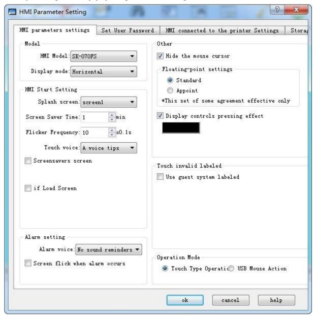
Figure 7-3 HMI Parameter Setting dialog box
