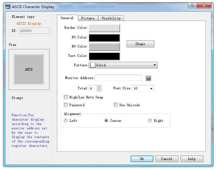
Figure 4-99 ASCII Display dialog box
