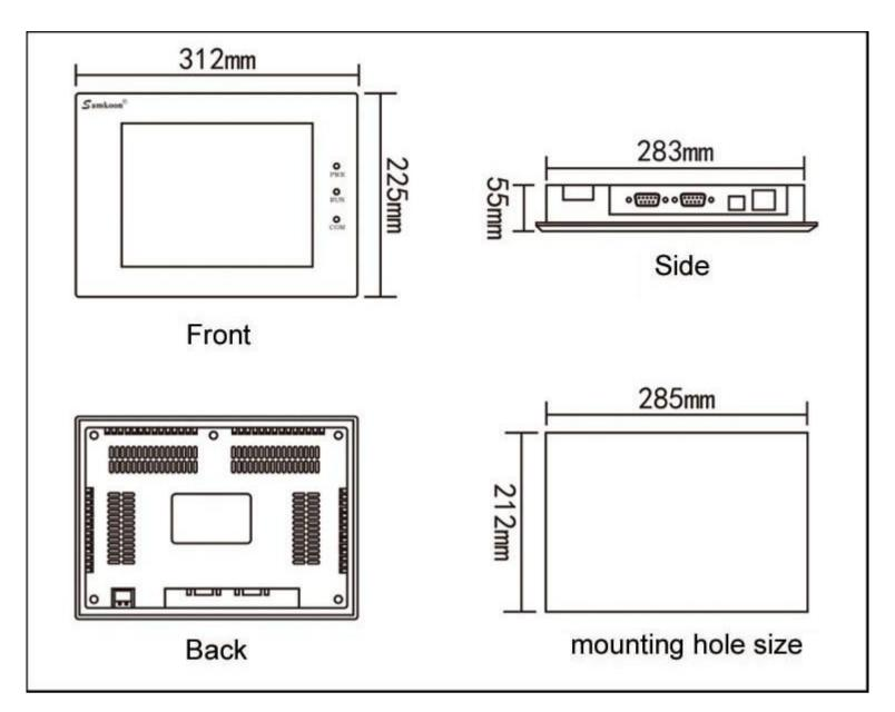
Figure 1-9SK-104F mounting dimension
