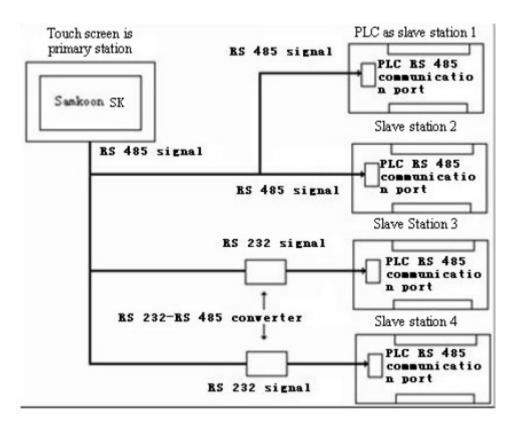
Figure 8-8 "One screen with multiple machines" connection
