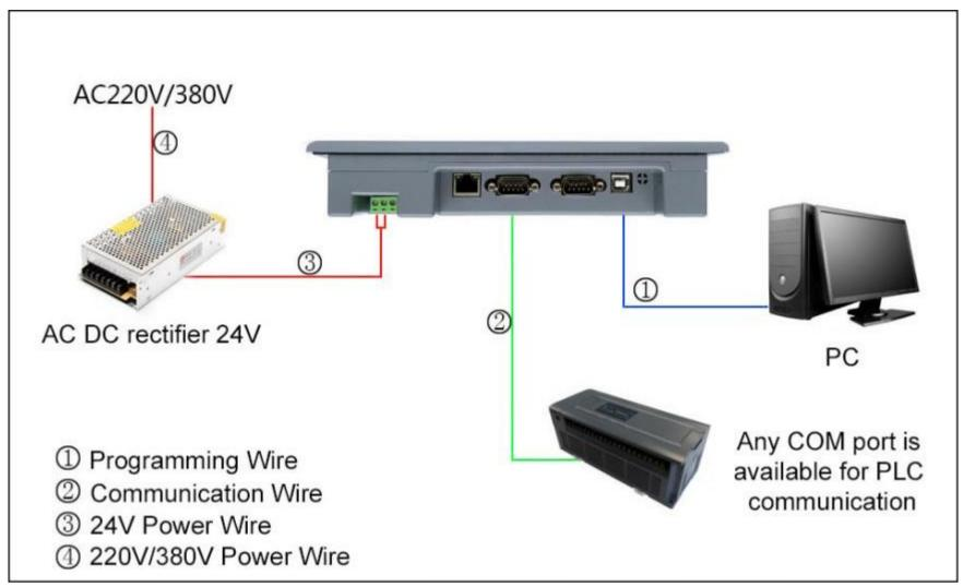
Figure 1-18 Connection diagram of SK series touch screen
