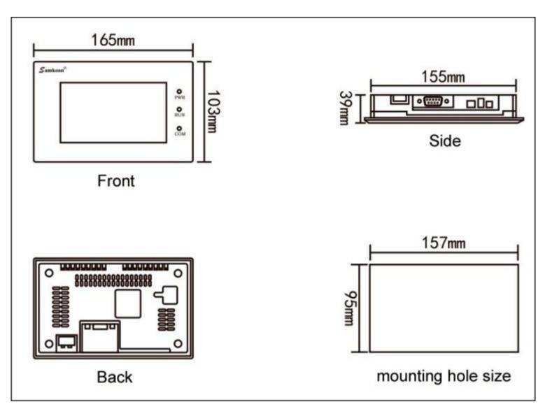
Figure 1-4 SK-050H mounting dimension
