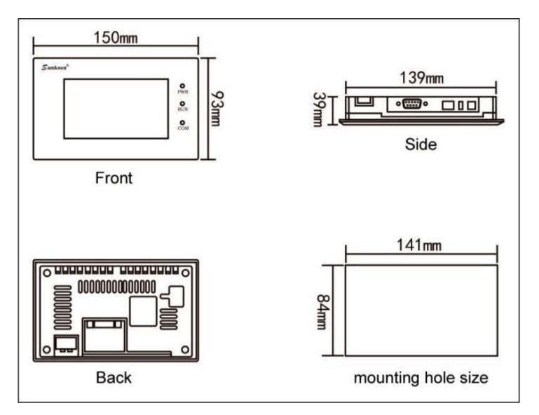
Figure 1-2 SK-043FE mounting dimension
