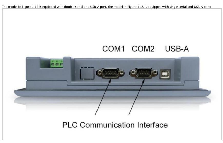
Figure 1-14 Side panels of SK ( double serial )
