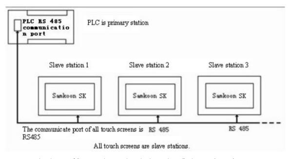
Figure 8-4 Sketch map of "One machine with multiple machines" when PLC(RS485) is Master station
