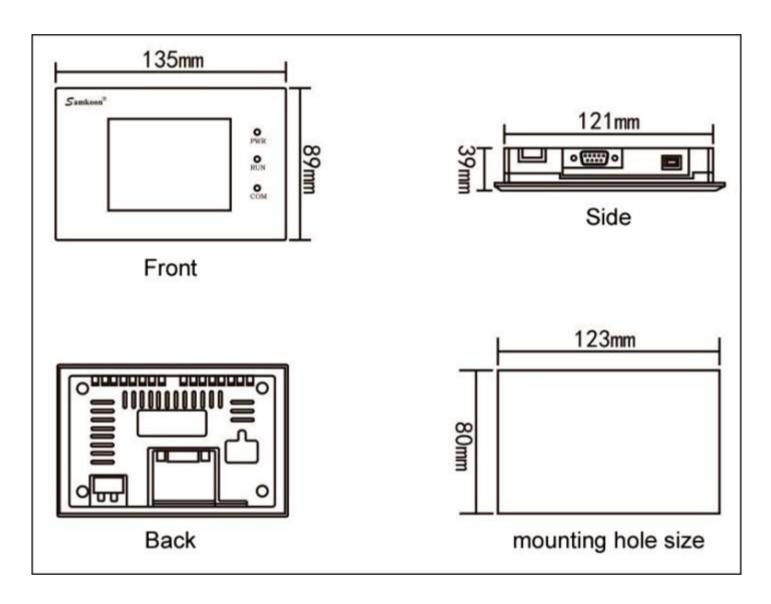
Figure 1-1SK-035FE mounting dimension
