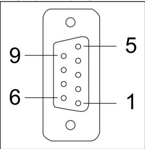
Figure 1-16 9-pin communication port
