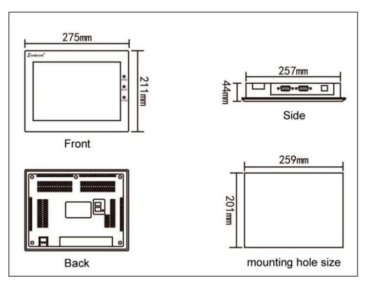
Figure 1-8 SK-102H mounting dimension
