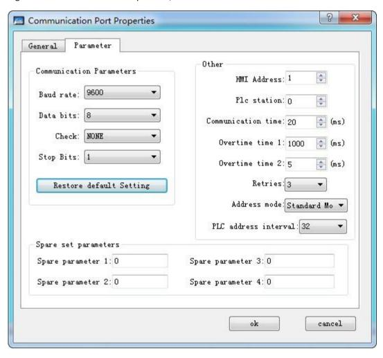
Figure 8-3 Allocation station address of HMI
