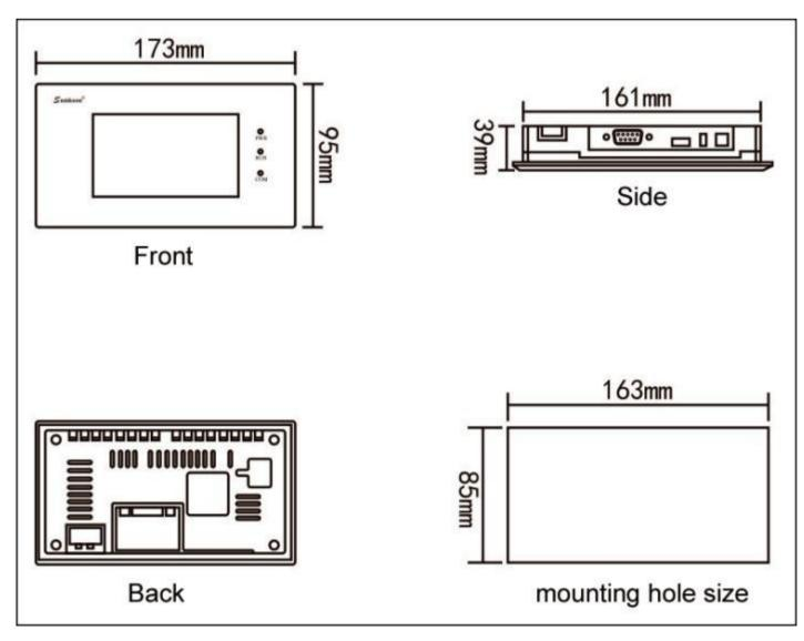
Figure 1-3 SK-043HS/SK-043HE mounting dimension
