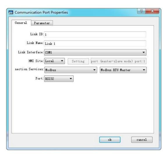
Figure 8-9 Set the touch screen as Master Station
