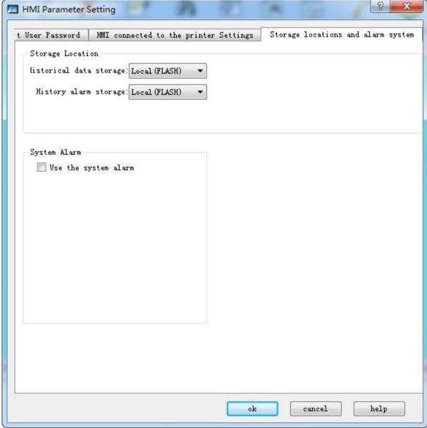
Figure 7-6 Storage location and Alarm system
