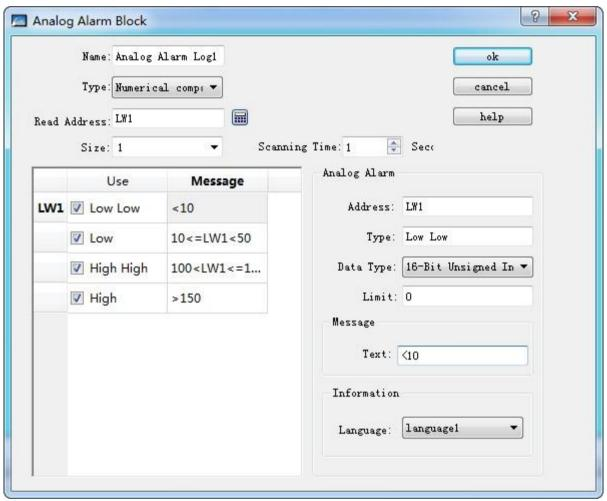
Figure 7-28 Analog Alarm Login dialog box
