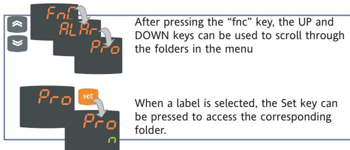
After pressing the “fnc” key, the UP and DOWN keys can be used to scroll through the folders in the menu
