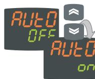
To change the status of a function, use the UP and DOWN keys.
