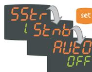
The label will be displayed, with the current status of the function. To scroll through the available functions, use the Set key.
