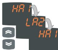
If there are alarms present, the UP and DOWN keys can be used to scroll through and display them
