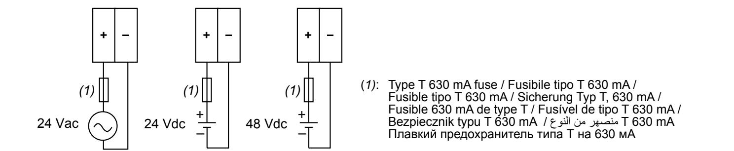
The power supply terminals and the signal reference for CAN (indicated as GS connections) are not internally connected /
