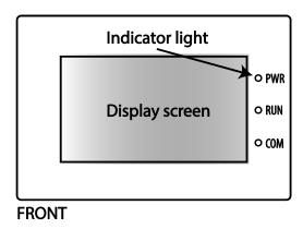
Figure 1-14: Front panel of TGI series
