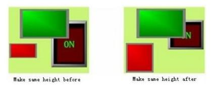
Figure 4-22: Contrast before and after "The Same Height"
