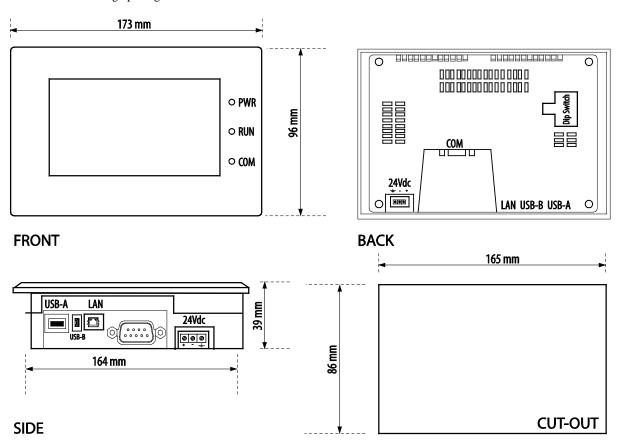
Figure 1-2: Installing dimensions of TGI SK043S/B
