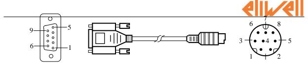
TGI series touch screen uses DB9F connector. Delta DVP series PLC terminal is MD8M.
