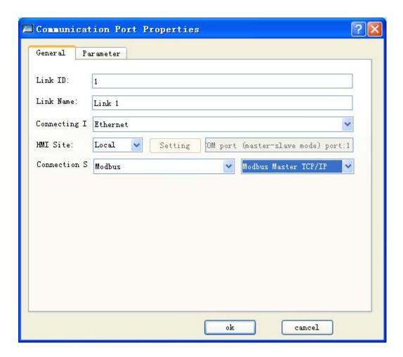
Figure 8-20: Ethernet connection and modbus TCP/IP protocol
