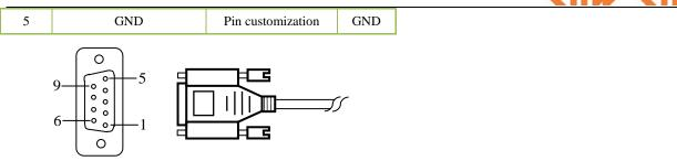
TGI series touch screen uses 9P trapezoid female-connector. The pin at AIBUS device terminal is defined as AIBUS device.
