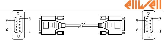
TGI series touch screen uses DB9F connector. Nanda NA-200/400 series PLC terminal is DB9M.
