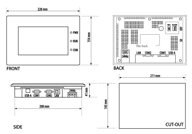
Figure 1-7: Installing dimensions of TGI SK07AS
