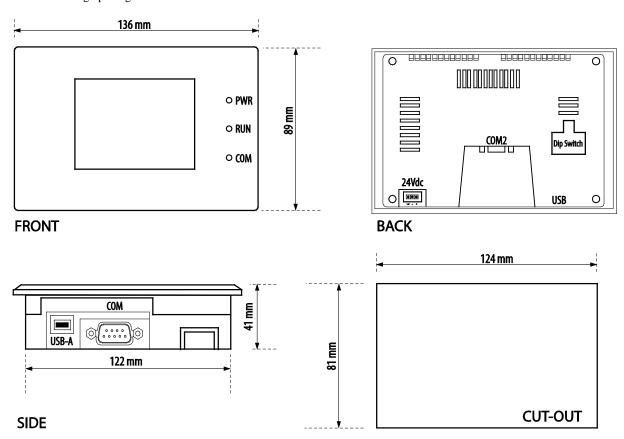
Figure 1-1: Installing dimensions of TGI SK035AE
