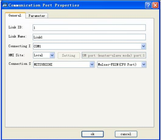
Figure 8-18: General page of property setting for remote HMI communication port
