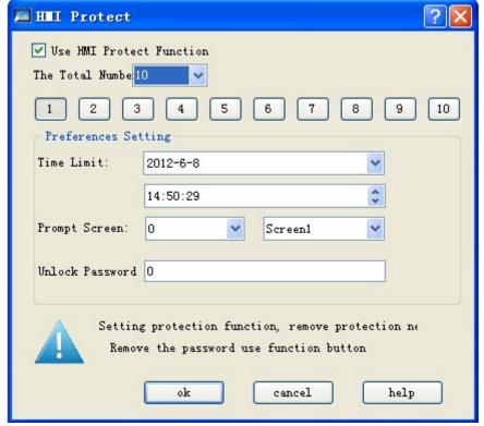
Figure 7-12 Dialog box of HMI protect
