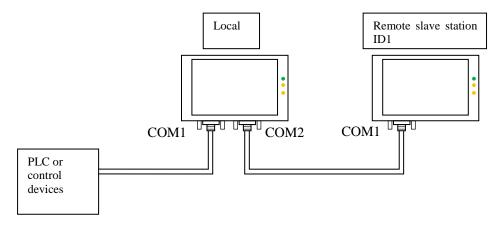
Figure 8-12 connection diagram of two-screen penetration
