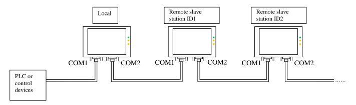
Figure 8-13 connection diagram of multi-screen penetration
