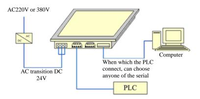
Figure 1-18: Connection diagram of TGI series touch screen
