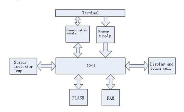
Figure 1-17: Schematic diagram for the structure of TGI series touch screen
