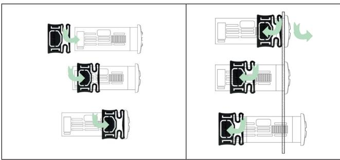
Fig. 4. Example of panel mounting - side view
