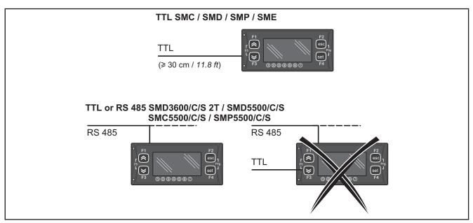
Fig. 21. Serial connection: TTL / RS485
