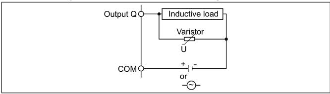
Fig. 20. Protective circuit C
