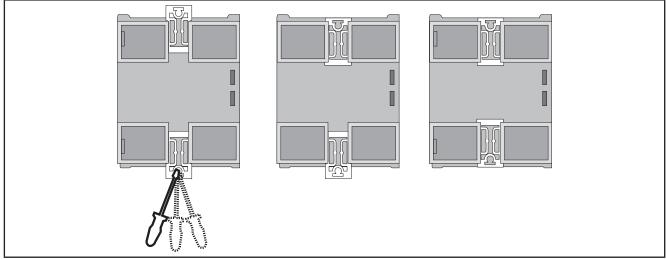
Fig. 7. Installation on DIN rail – rear view
