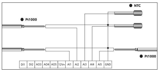
Fig. 30. Pt1000 input connection
