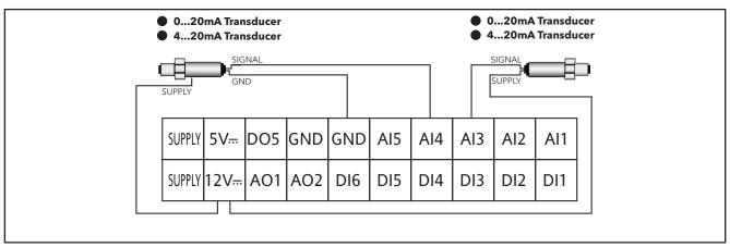
Fig. 27. Current input connection
