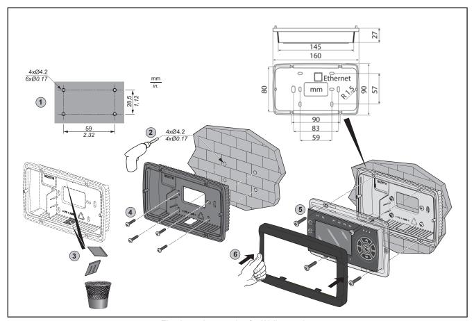
Fig. 15. Accessories for Wall mounting
