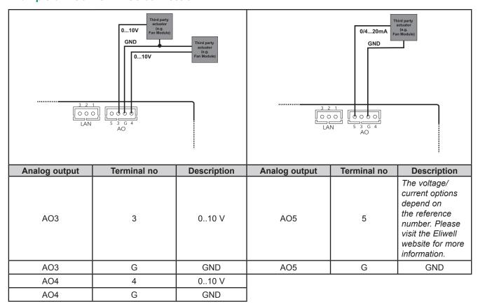
**Fig. 34.** Example of SMP connection (AO3-AO4) with 1 0...10 V fan module
