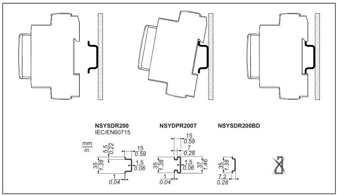
Fig. 6. Installation on DIN rail – side view
