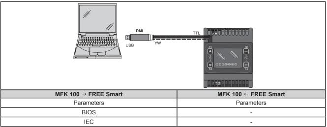
Fig. 54. Connections between MFK 100 and the FREE Smart
