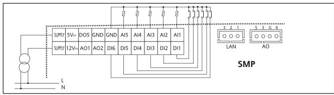
Fig. 31. SMP - Example of low voltage input / output connection
