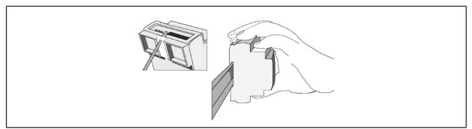
Fig. 8. Installation on DIN rail  $-\frac{3}{4}$  view
