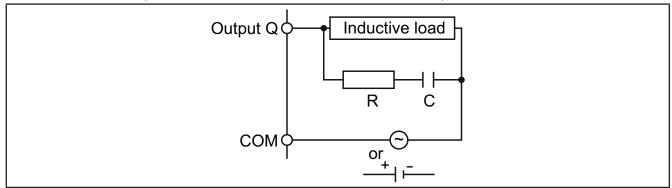
Fig. 18. Protective circuit A
