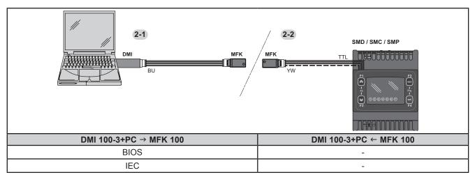
Fig. 55. Connections between MFK 100 and DMI 100-3 + PC
