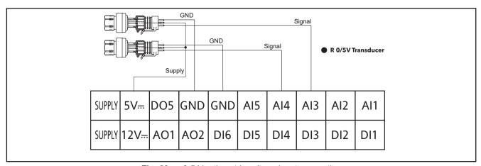
Fig. 29. 0-5 V ratiometric voltage input connection
