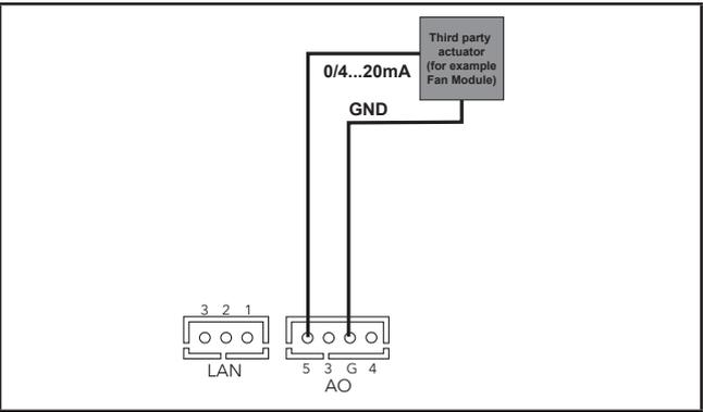
**Fig. 22.** Example of EWCM 436D PRO / A-CR11 (AO5) connection with 1 0...20 mA / 4...20 mA fan module
