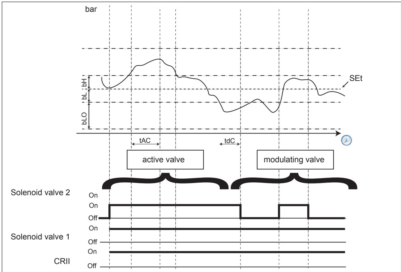
Fig. 33. Valve switch-off mode
