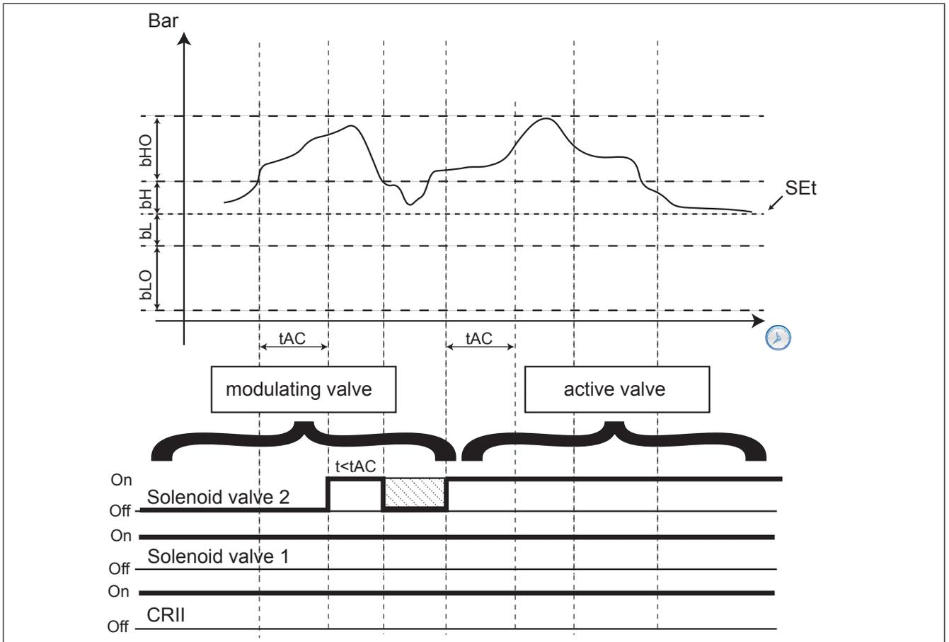
**Fig. 32.** TC2 from modulating to active
