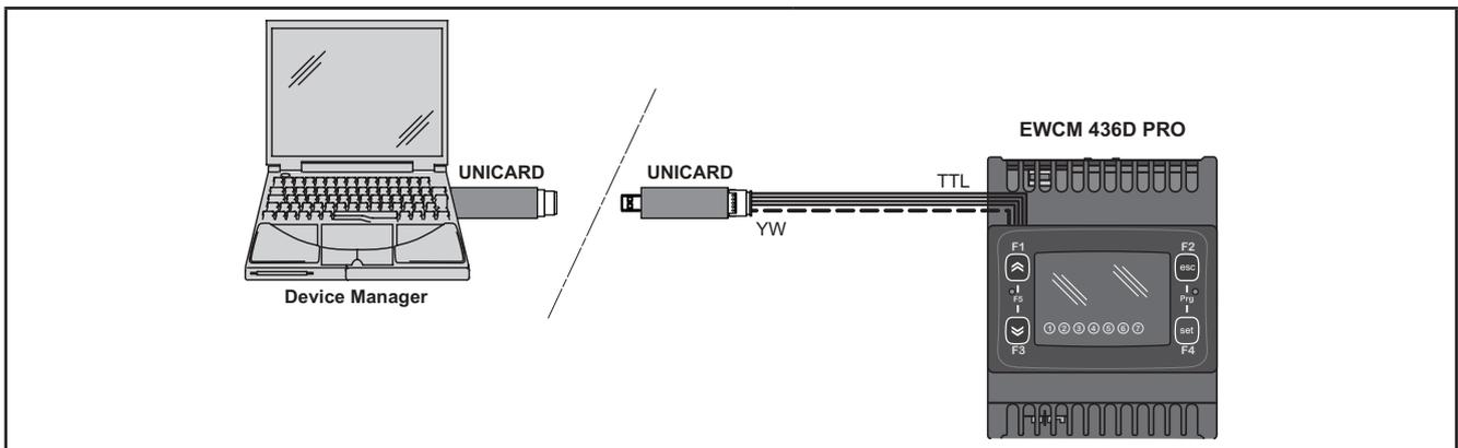
**Fig. 40.** Connection between UNICARD and Device Manager + EWCM 436D PRO
