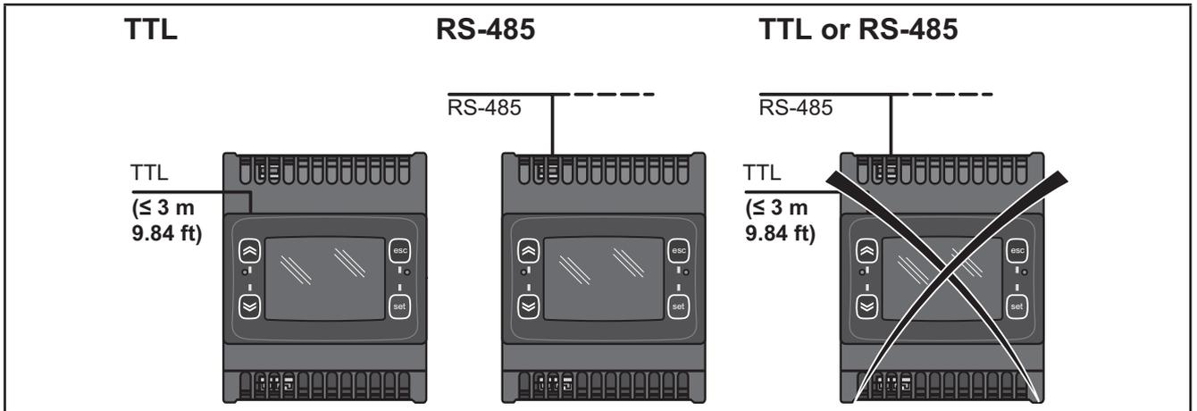
Fig. 13. Serial connection: TTL / RS485
