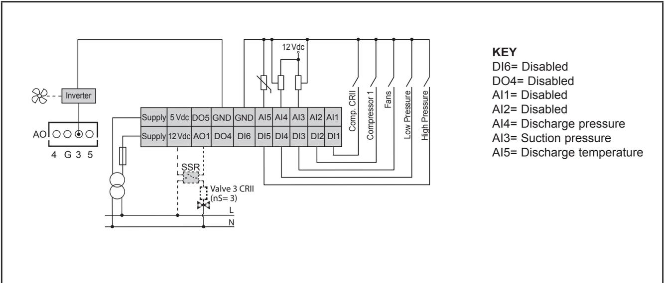
Fig. 24. Standard configuration of digital/analog inputs
