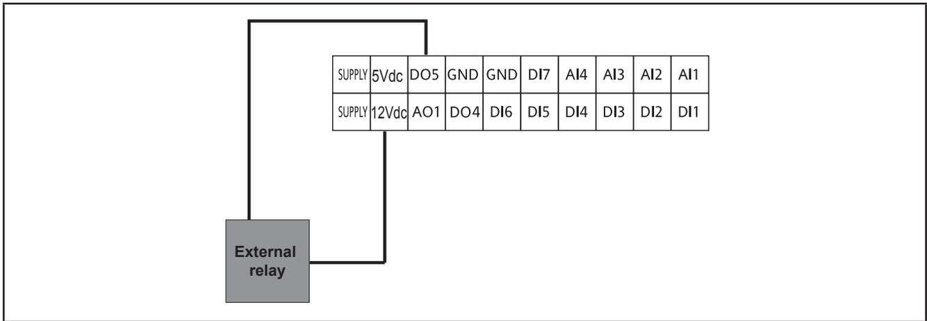
**Fig. 23.** Example of DO5 connection with an external relay
