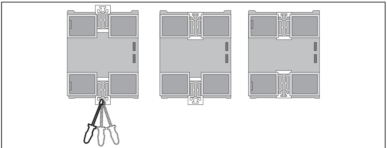
Fig. 3. DIN rail installation - rear view
