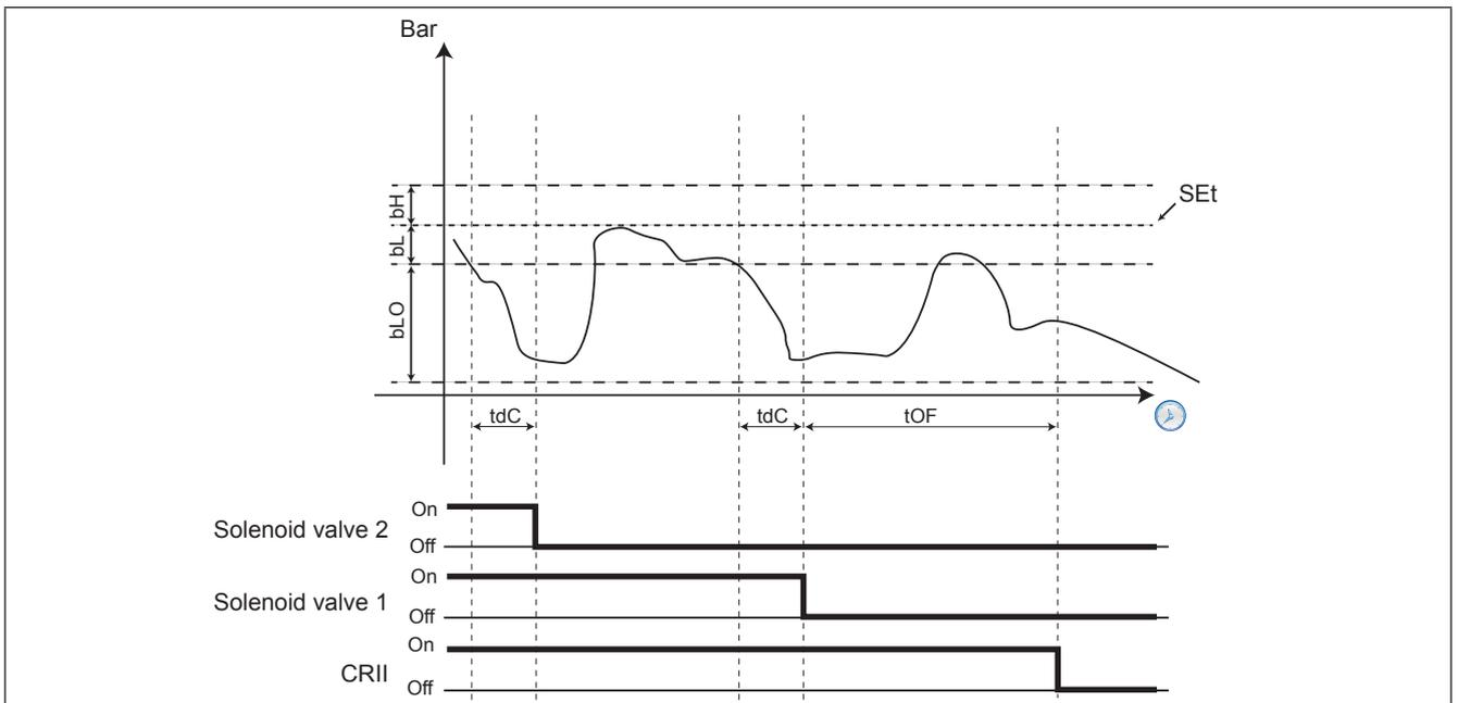
Fig. 34. Switching off the CRII compressor
