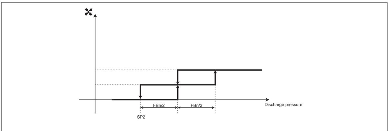
**Fig. 35.** Enabling the digital fans
