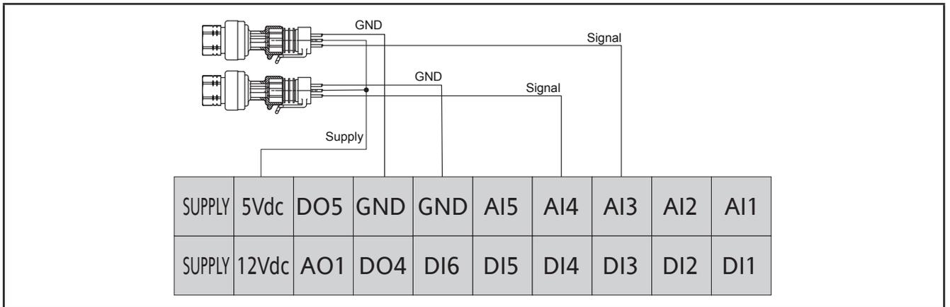
Fig. 18. Voltage connection of ratiometric inputs 0...5 V
