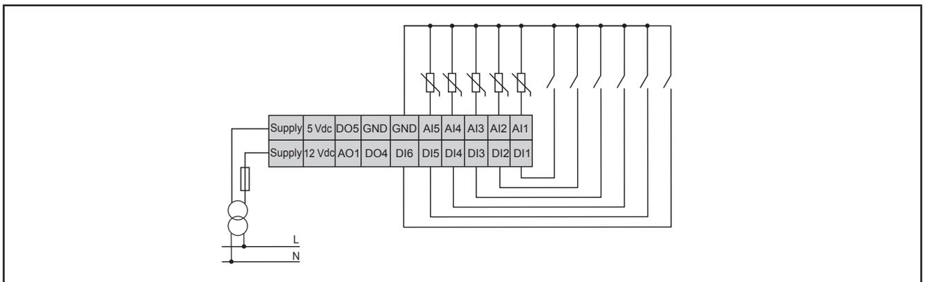
Fig. 19. Example of analog/digital input connection
