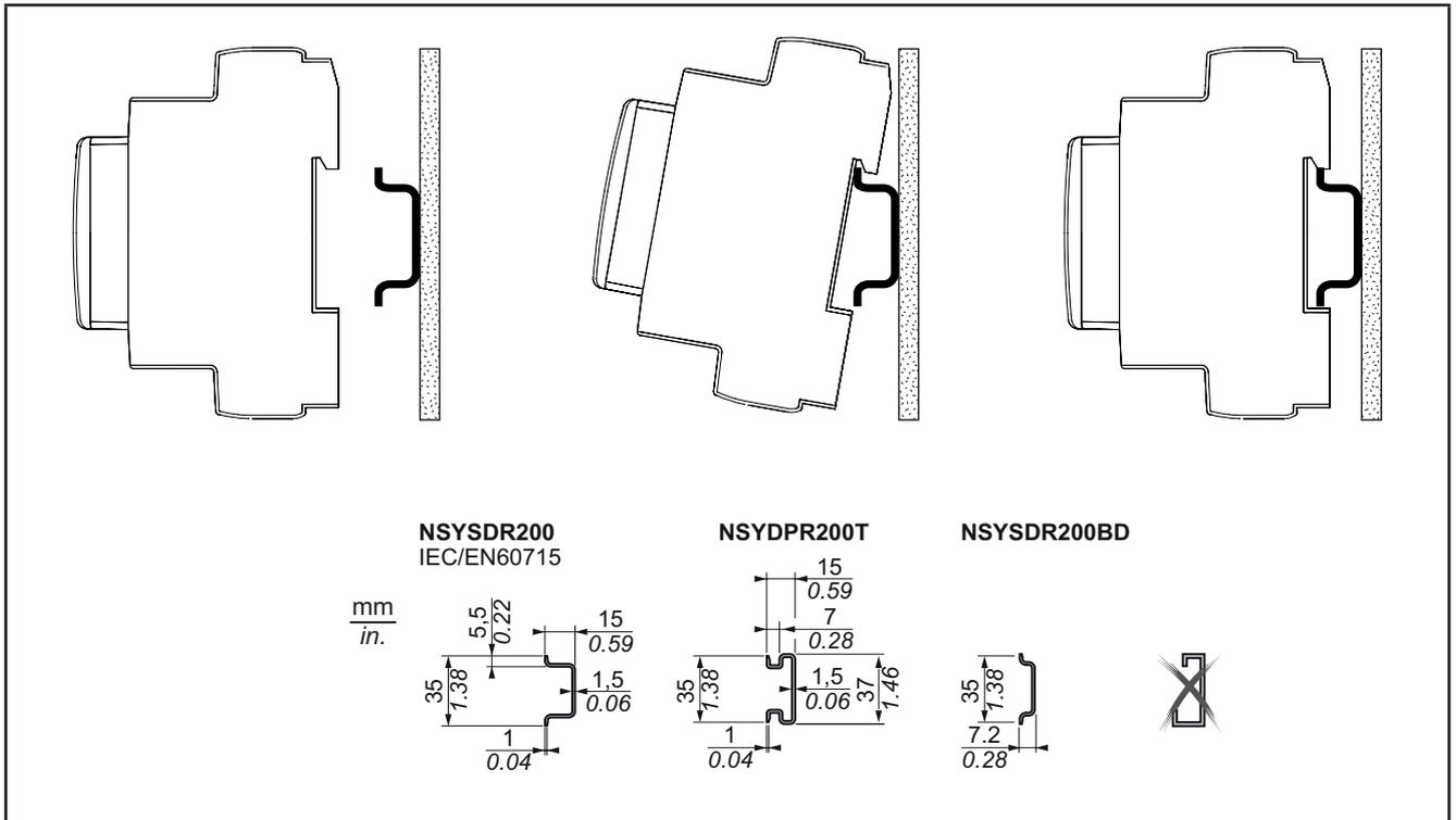
Fig. 2. DIN rail installation – side view
