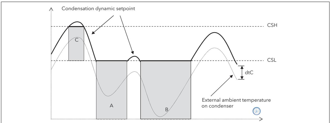
Fig. 36. Floating condensation
