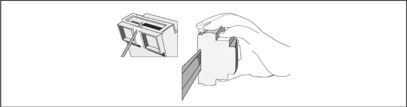
Fig. 4. DIN rail installation – ¾ view
