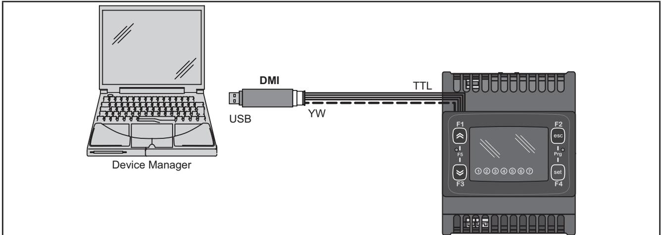
Fig. 38. Connection between **DMI / UNICARD** and **EWCM 436D PRO**
