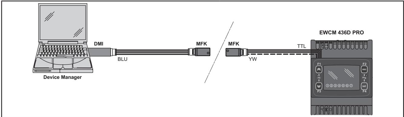
**Fig. 39.** Connection between the MFK/UNICARD and DMI + Device Manager
