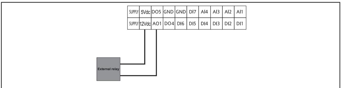
Fig. 20. Example of AO1 connection with an external relay
