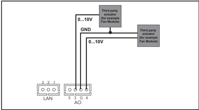
**Fig. 21.** Example of EWCM 436D PRO / A-CR11 (AO3-AO4) connection with 1 x 0...10 V fan module
