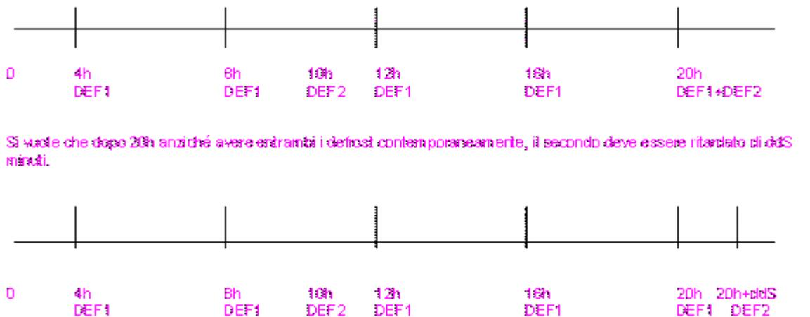
At the twentieth hour the two defrosts occur at the same time, even if the "non-simultaneous" option was set. To avoid this, set  $ddS$  to a value other than 0 (Range  $ddS$ : 0..60 min).
