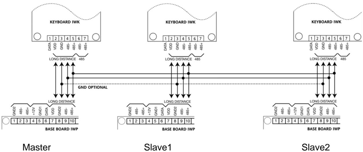
Link connection in case of IWK keypad Short distance connection
