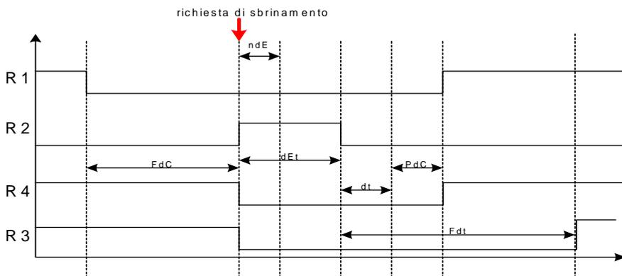
The end of defrost, for the probe (in respect of parameter  $ndt$ ) or for timeout (par. $dEt$ ), will be followed by dripping (par. $dt$ ) after which the device returns to normal operating conditions and therefore the possibility of activating R4 if required by the temperature controller and R1 after par.  $PdC$ .
